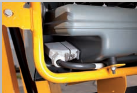
The electrical connectors of the upper control box are easy to connect and offer excellent water resistance
