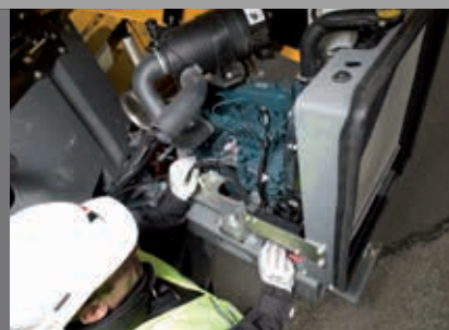
Swing out engine tray enabling direct access to key components
