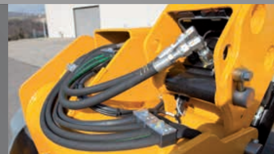
Close up of the boom hydraulic routing
